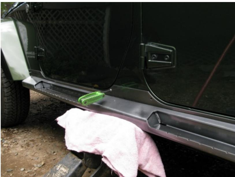
Lift the rocker back into place. Tighten the 5 1/4"x1" allen bolts into the nut zerts. Use a med strength thread locker on the 6 5/16"x 1" bolts then tighten them thru the bottom of the rocker into the rocker support.
