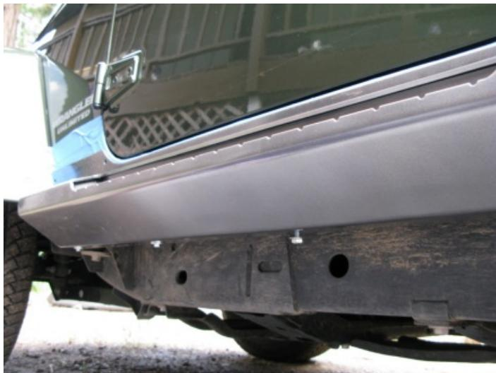
Mask off the area of the car that the rocker will come in contact with including the fender flares. Lift the the rocker into place. Bolt in place using 6 of the 5/16"x1" bolts with a flat washer on each. Hand tighten all of the bolts. Make sure that the rocker is centered on the doors. Once centered tighten the bolts.
