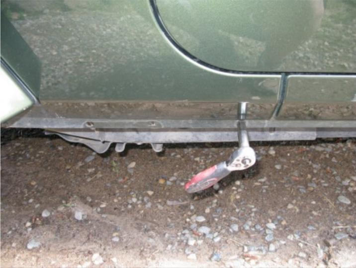
Remove the factory fender bolt using a 10mm.
