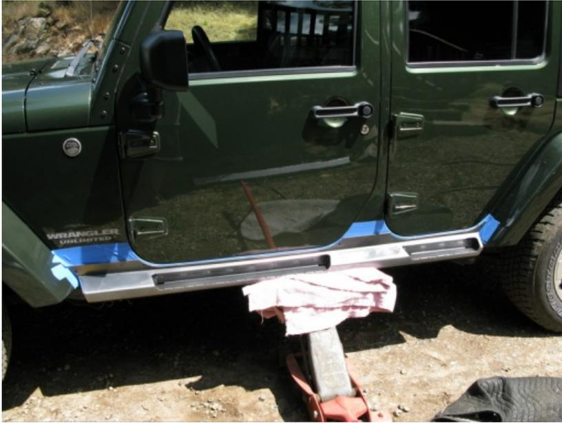
Using a floor jack with a block of wood wrapped in a towel, jack on the out side of the rocker pushing it tight against the jeep. Recheck your alignment and recenter if necessary.
