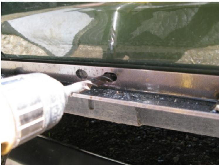
Using a 3/8" drill bit, drill the remaining holes thru the pinch weld using the rocker support as a guide.
