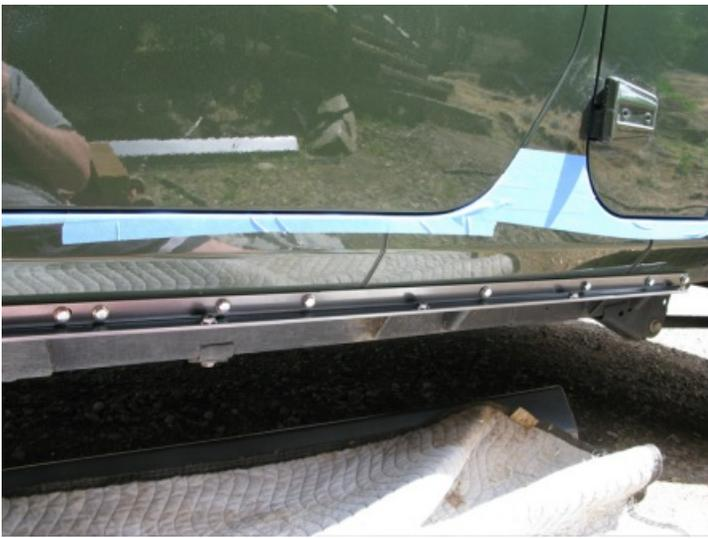
Install the 5/16"x1" bolt with a flat washer thru the rocker support. Tighten the 5/16" nylock with a flat washer on the back side of the pinch weld. When finished you should have 11 5/16" bolts installed and the one factory fender bolt.
