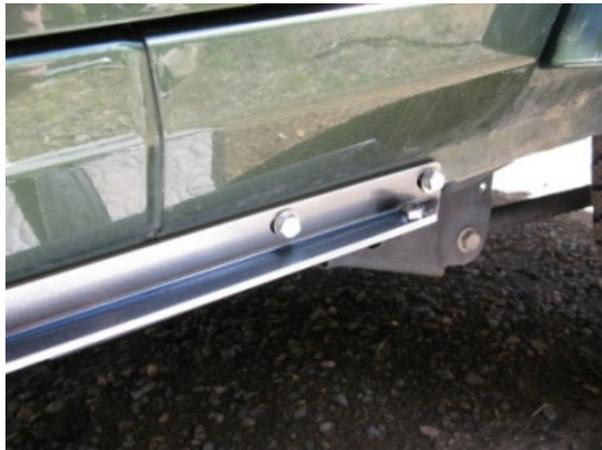
Find the rocker support that matches the holes in the pinch weld. Using the factory fender bolt you just removed and the supplied 5/16"x1" bolts mount the rocker support. Insert the 5/16"x1" bolts with a flat washer thru the rocker support. Tighten the 5/16" nylock with a flat washer on the back side of the pinch weld. Do this to all of the bolts that align with a hole on the pinch weld.
