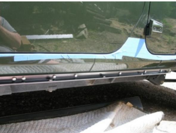
Install the 5/16"x1" bolt through the rocker support. Tighten the 5/16" nylock with a flat washer on the back side of the pinch weld. When finished you should have the supplied 5/16" bolts installed and the one factory fender bolt.
