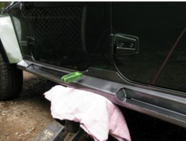
Lift the rocker back into place. Tighten the 1/4"x1" allen bolts into the nut zerts. Use a med strength thread locker on the 5/16"x 1" bolts then tighten them through the bottom of the rocker into the rocker support.
