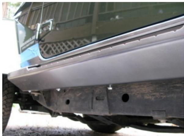
Mask off the area of the car that the rocker will come in contact with including the fender flares. Lift the the rocker into place. Bolt in place using the 5/16"x1" bolts . Hand tighten all of the bolts. Make sure that the rocker is centered on the doors. Once centered tighten the bolts.
