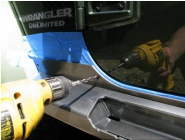
Using a 1/4" drill bit with a center punch carefully pilot at the very center of all 5 holes along the top of the rocker. On the two forward holes be sure to pilot through the second inner layer. Once all of the holes are drilled remove the rocker from the jeep.
