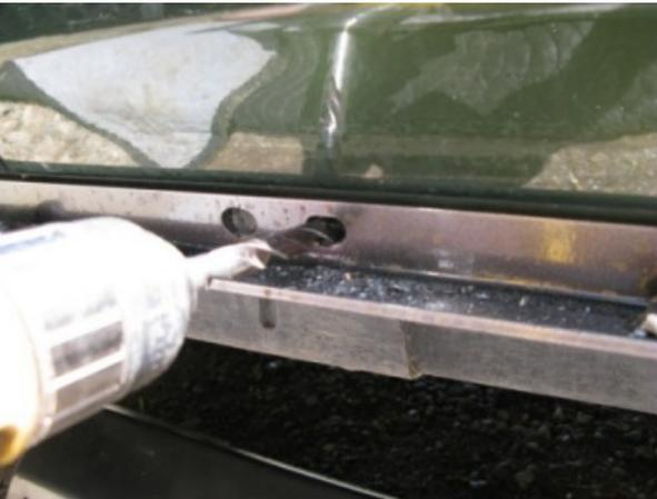
Using a 3/8" drill bit, drill the remaining holes thru the pinch weld using the rocker support as a guide.
