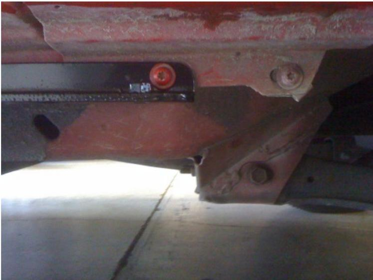
1. Install lower mount rail to the body of the Cherokee as shown.
