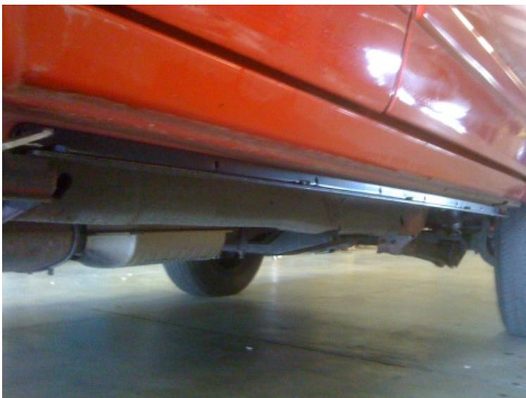
2. With the rail snugly in place. Install the rocker and align along the body.
