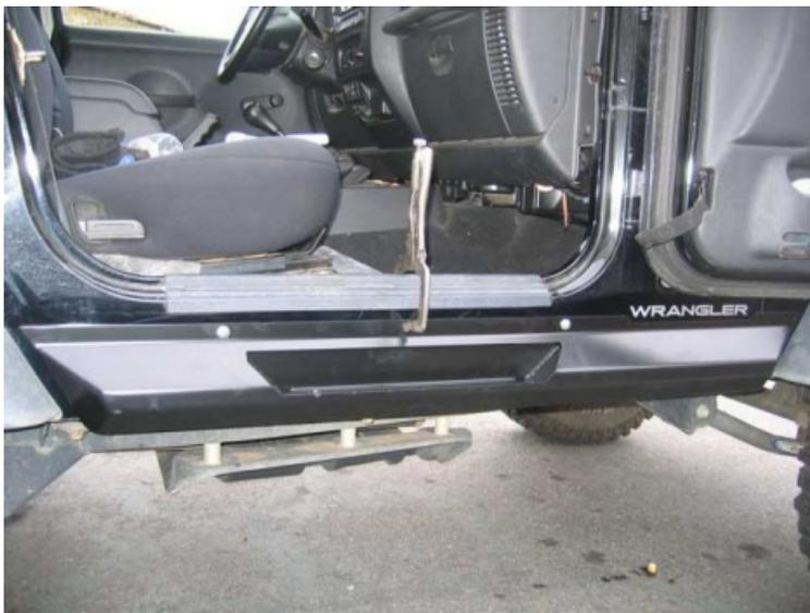
3. With the rocker in place, transfer all holes along the body to be drilled.
