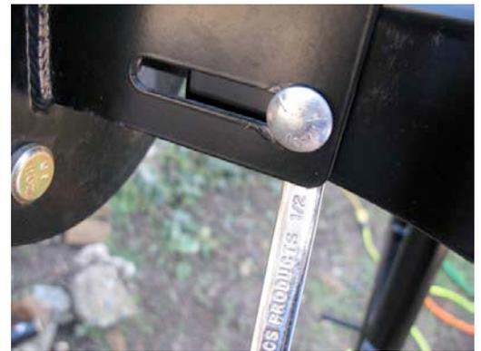
Insert grease fitting and thread in using a 5/16" wrench.
