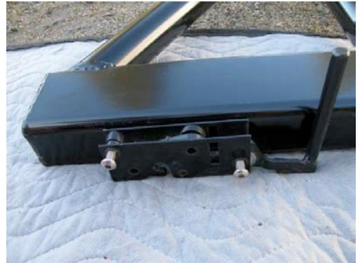
Install the detent stud with the supplied spring on it. Lube the detent before installing.
