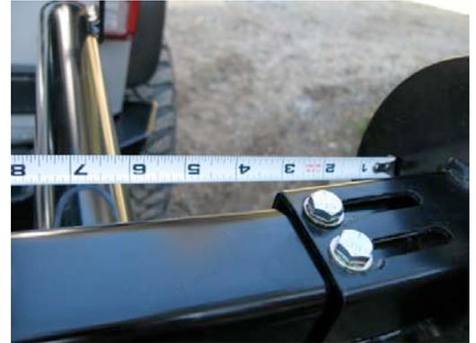
Insert two 5/16"x3/4" carriage bolts, use flat washer and 5/16" nylock nuts. Tighten with 1/2" wrench.
