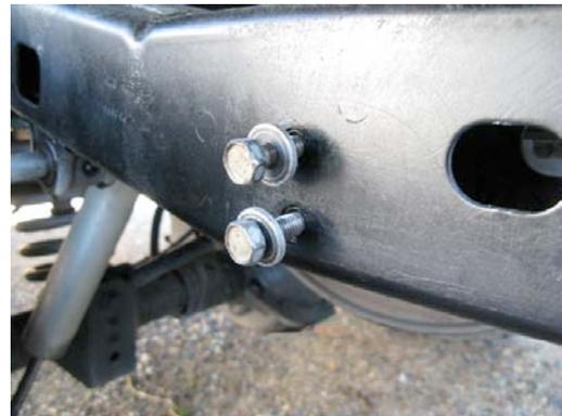
There are four holes in the back of the frame. You will need to enlarge the far right hole using a drill with a 9/16" metal bit.
