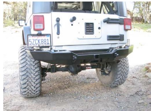
Install the 4 bolts you retained from your stock bumper 2 into each side of the frame. Hand tighten.
