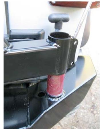
Work the tire carrier back and forth until the tire carrier is all the way down onto the spindle.
