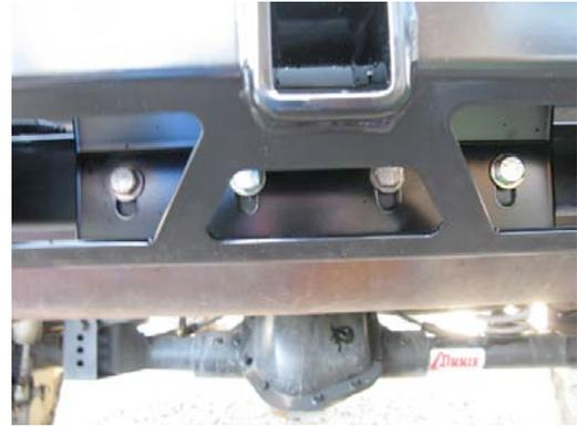
Adjust bumper making sure the top is running parallel with the ground. Stand back and make sure it is aligned with the back of the vehicle.
