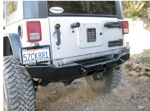
Tighten the bolts into the side of frame using a 16mm socket.
