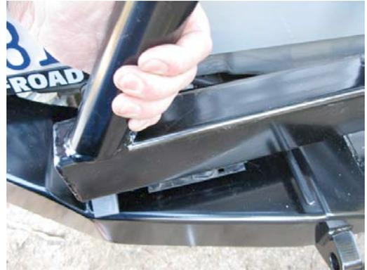
With the tire carrier in the closed position insert the 2@ 5/16" x 1 1/4" bolts thread on the c-nuts(self locking). Tighten the nuts until snug. Do not over tighten, the clamp sleeve should not touch it self. Test tightness by opening the tire carrier carefully. The tire carrier should not droop to hit the bumper. Work tire carrier back and forth and readjust if necessary.
