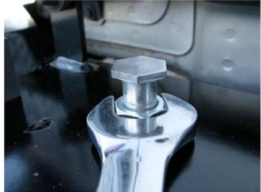
Insert the 2 @  $\frac{1}{2}$ " x  $1\frac{1}{2}$ " bolts with a flat washer and nut locking into position. Hand tighten.
