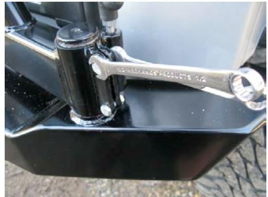
With the tire carrier closed, check for latch alignment.
