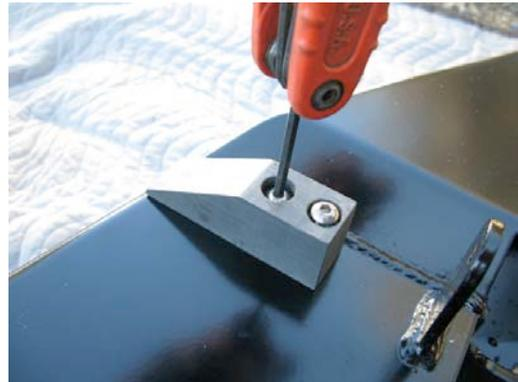
Insert the latch pin into the bumper. Install with nut and washer on top of the bumper and flat washer, lock washer and nut from under the bumper. Only hand tighten at this time.
