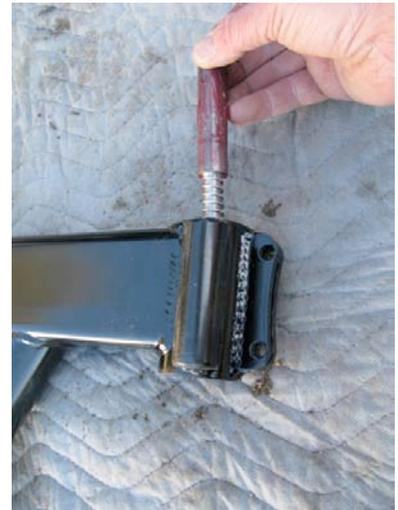
Thread on the  $\frac{7}{16}$ " nut and the tee handle. Tighten the nut against the tee handle to lock the tee handle in place.
